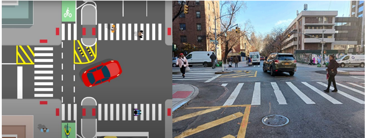
Figure 8 Bike Island Channelization Box (Source: NYC DOT, 2024)
