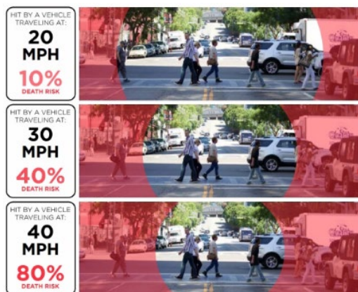
Figure 13 The effect of speed on a driver's field of vision and the risk of pedestrian fatality (LADOT, 2015)
