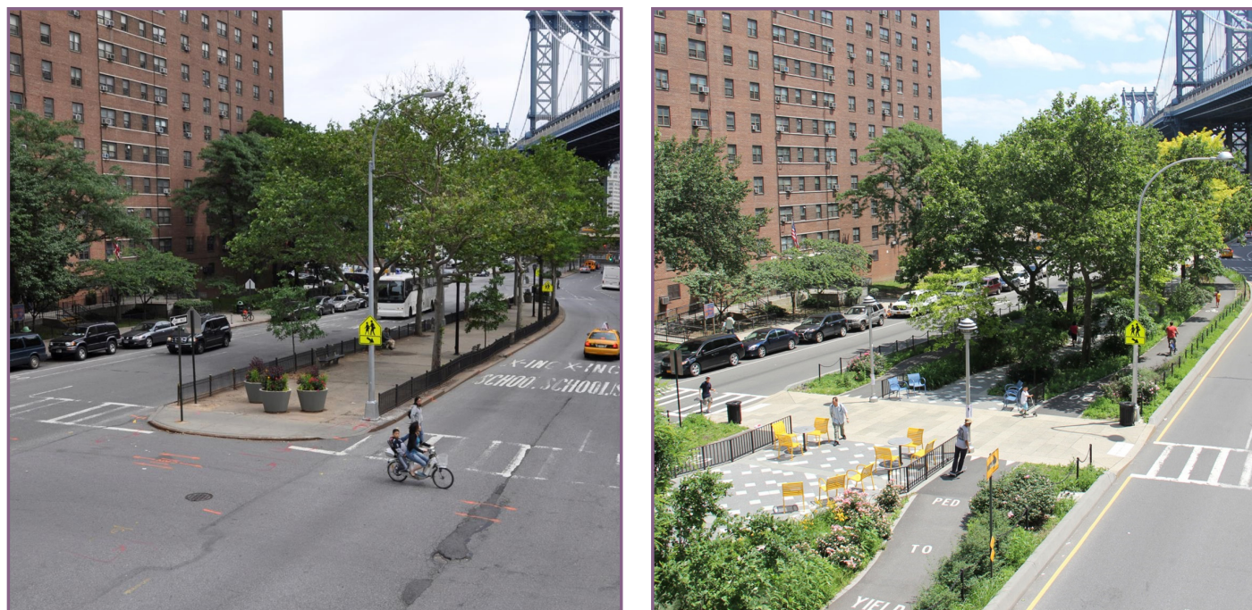
Figure 23. Medians can be widened to accommodate pedestrian- and bicyclist-oriented infrastructure like wider sidewalks, seating, pedestrian-scale lighting, bicycle lanes, and street trees. ( National Association of City Transportation Officials [NACTO] and the New York City Department of Transportation [NYCDOT] )
