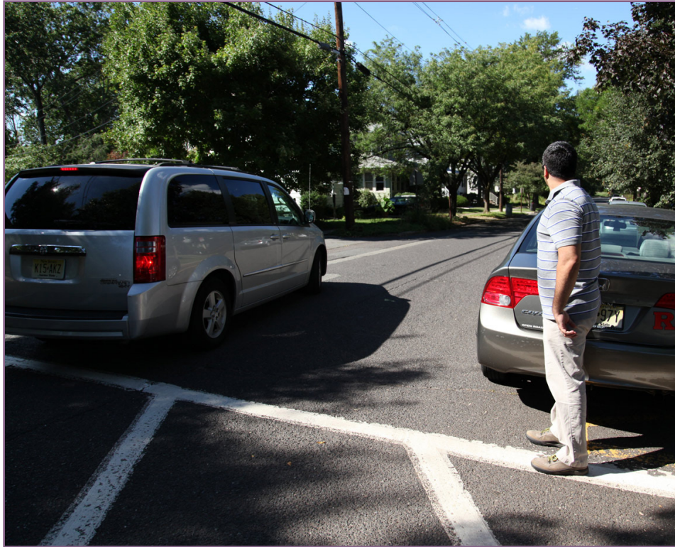
Figure 20. Parking restrictions on crosswalk approaches can improve sightlines for motorists and pedestrians. New Jersey law prohibits parking within 25 feet of a crosswalk and 50 feet of a “stop” sign. ( NJDOT Bicycle and Pedestrian Resource Center )
